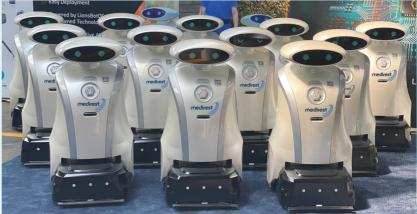
Designed to support Medirest's team of over 3,000 cleaners, the robots enhance repetitive cleaning procedures in open spaces such as corridors, freeing up other team members to focus on touch point and cross infection hot spots forming the perfect "cobotics" relationship.
